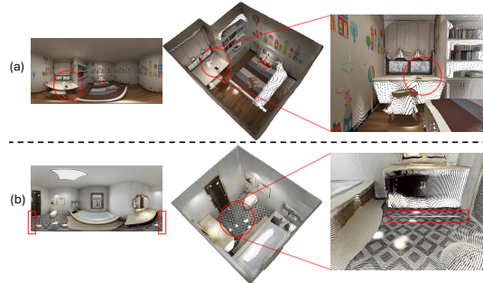
Figure 7: DA 2 ’s limitations. (a) The white lamp’s predicted distance is mistakenly aligned with the desk surface. (b) Visible seams appear along the predictions at lower left–right boundaries.
